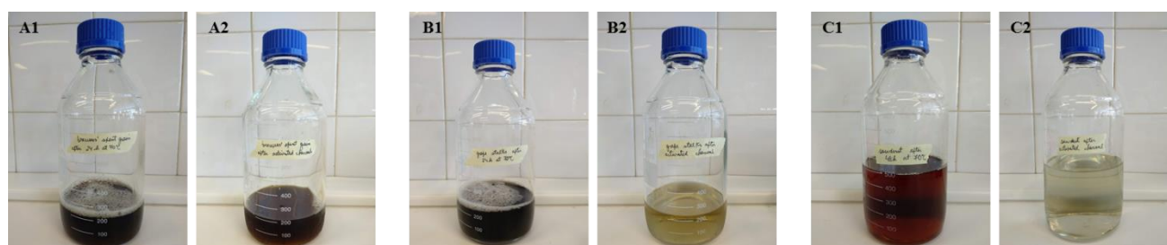
Figure 7 – Effect of activated charcoal on hydrolysates color. A1 – BSG before charcoal treatment; A2 – BSG after charcoal treatment; B1 – Grape stalks before charcoal treatment; B2 – Grape stalks after charcoal treatment; C1 – Sawdust before charcoal treatment; C2 – Sawdust after charcoal treatment.
