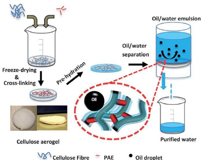
Figure 2. 1- Schematic of aerogels manufacture and application to oil/water separation. [46]
