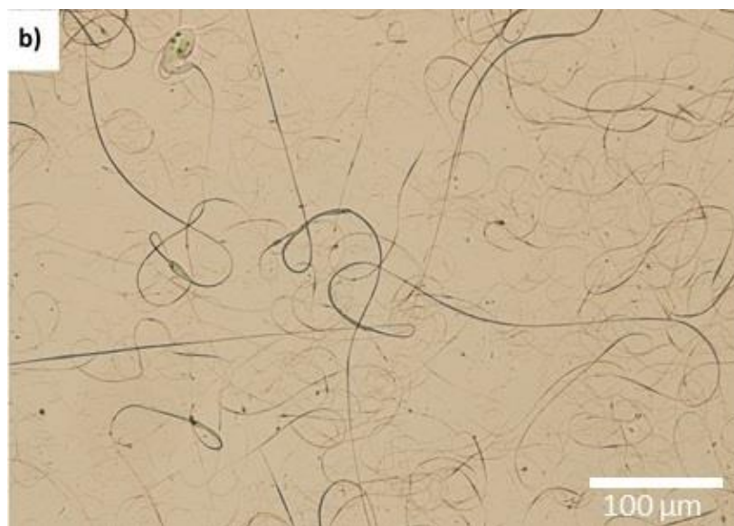
Figure 7. 2- POM images taken in transmission mode, between parallel polarizers, with a 50 \mu\text{m} magnification of CA/MMT nanofibers with less defects due to an optimized solution having yet some “beaded” and short nanofibers;
