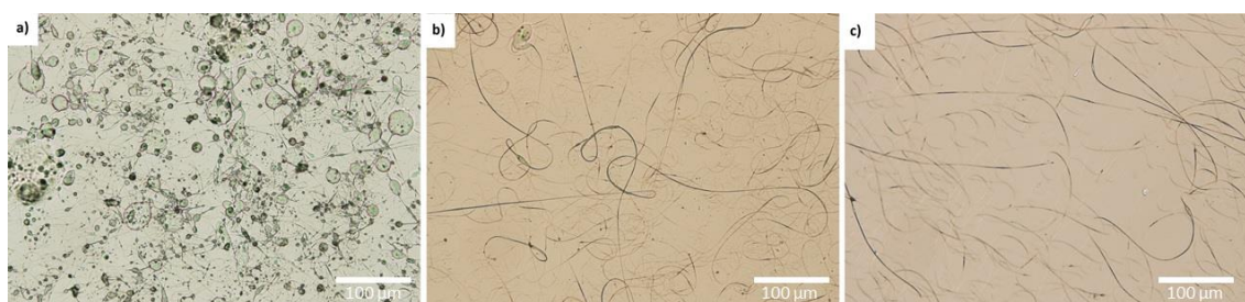
Figure 2.11- POM images of CA/MMT nanofibers taken in transmission mode between parallel polarizers with 50 \mu\text{m} magnification a) short and defective nanofibers derived from an inefficient solution and electrospinning parameters; b) nanofibers with less defects due to an optimized solution having yet some “beaded” nanofibers; c) optimized nanofibers with the final solution and electrospinning parameters.
