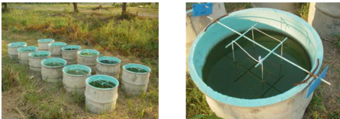
Figure 5 – Circular tanks used to set the microcosms (Source: Michiel Daam).
