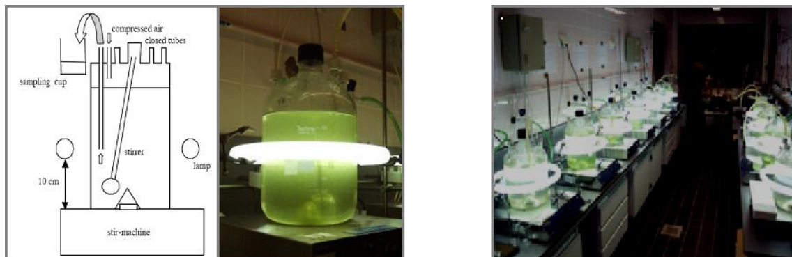
Figure 4 – Model Ecosystems used and predeposition (Source: Michiel Daam).
