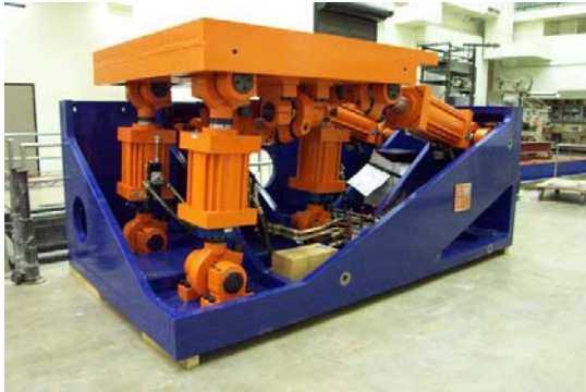
(a) Full-scale Load and Boundary Condition Box
