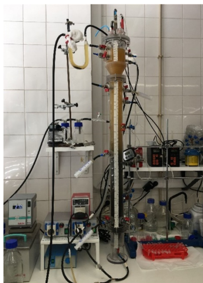
Figure 1. EGSB reactor used for the acidogenic fermentation of hydrolyzed BSG.
