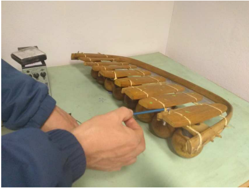
Figure 4.3: Experimental setup with impact hammer and accelerometer.
