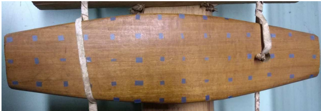
Figure 4.8: Experimental mesh for the complete modal analysis of bar # 4. The laser was pointed to the top left corner and impacts were given at all marked points of the mesh.
