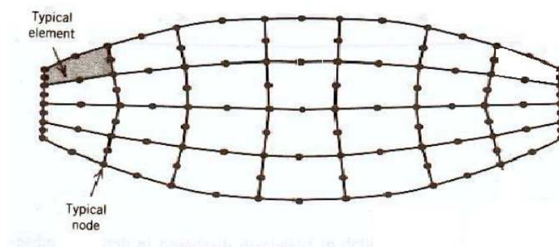
Figure 5.7: The timbila bar is divided into a number of elements connected by nodes.
