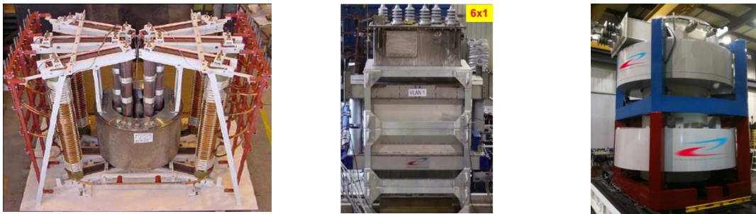
(a) 1 o Generation Prototype – the spider design. (b) 2 o Generation Prototype – Rectangular Compact SFCL. (c) Commercial Product – Round Compact SFCL.
