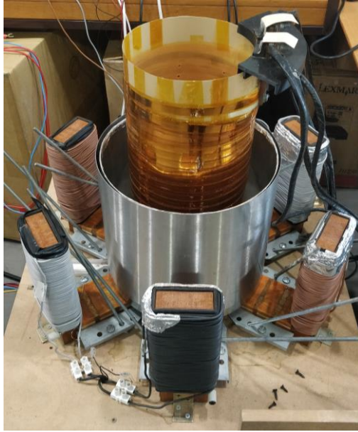
Figure 4.25 – Final assembly of the SC-SFCL.
