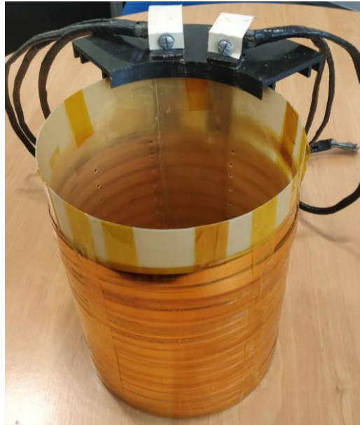
Figure 4.23 – DC bias coil and its support made of G11 material.
