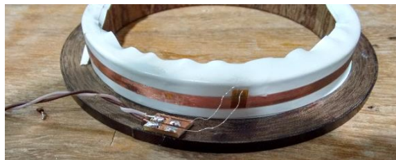
Figure 5.5 – Secondary winding (one HTS ring inserted into the winding holder).
