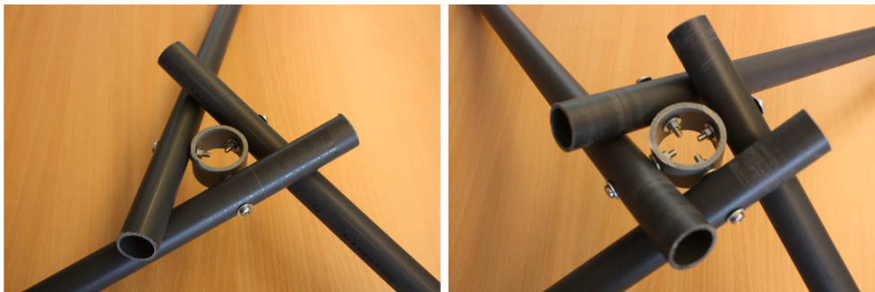
Fig. 3. Reciprocal linkages using three and four bars.
