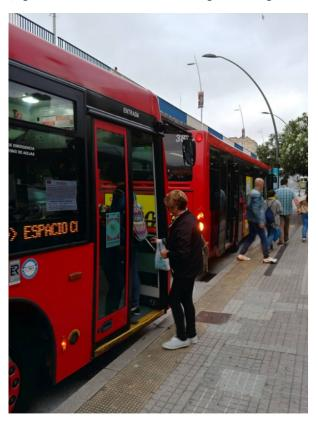
**FIGURE 1(d).** *Almost-level boarding and alighting*
