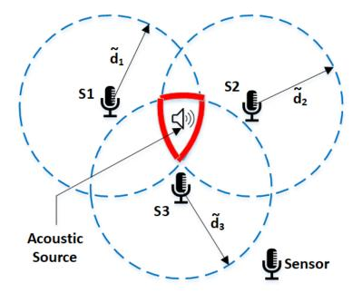
Figure 1. Sensors' distance estimate representation when measurement noise is considered.
