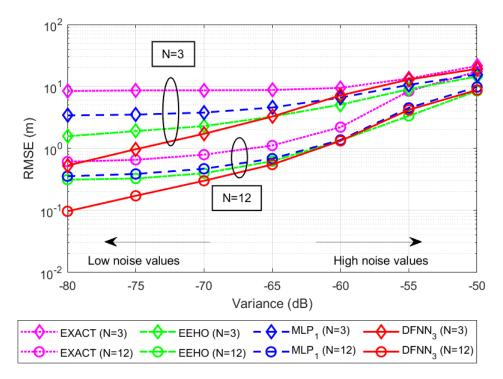
**Figure 8.** RMSE Comparison of *EXACT*, *EEHO*, *MLP*<sub>1</sub>, and *DFNN*<sub>3</sub> for N = 3 and N = 12.
