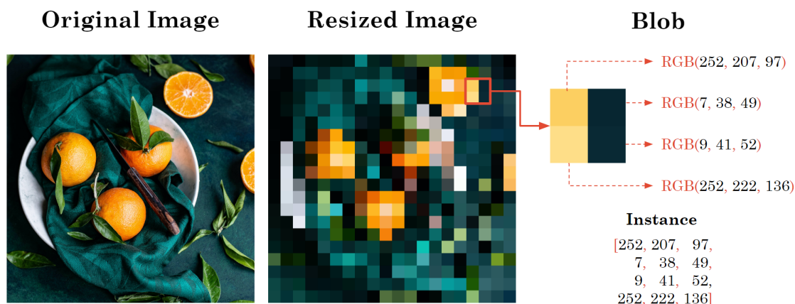
Figure 3.4: Representation of the Single Blob with No Neighbors Bag Generator [37] methodology. The original image is resized (in this example to 20 \times 20 pixels) and later split into 2 \times 2 pixels blobs. The features of the instance associated with each blob are the RGB values of its pixels.
