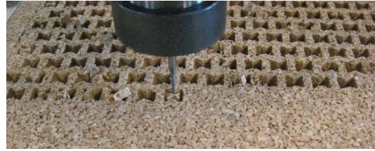
Figure 40 Making of the auxetic core
