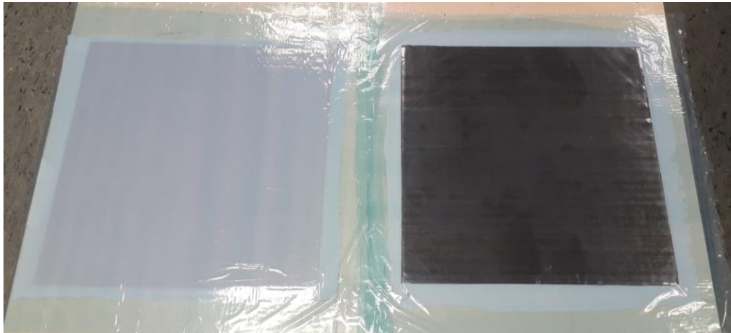
Figure 35 Skins are ready to go to the hot press. On the left the top side has the bleeder fabric and plastic release agent; on the right, the top side just has the plastic
