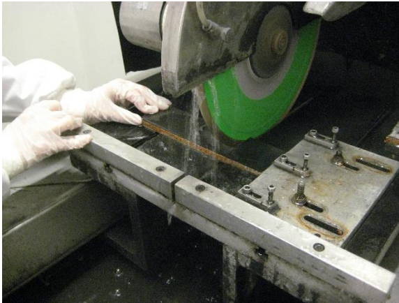
Figure 45 Saw used to cut the test specimens
