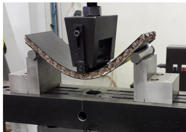
Figure 47 Three-point bending test specimen configuration, during the test
