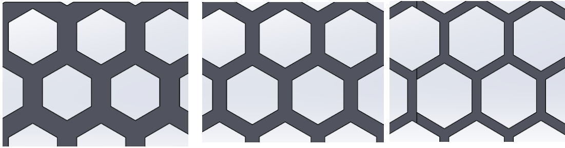
Figure 20 Structure Display: from the left to the right: structure 1 , D10 [mm], thickness 2 [mm]; Structure 2: D11 [mm], thickness 1.5 [mm]; Structure 3, D12 [mm], thickness 1 [mm]
