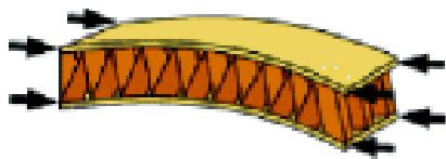
Figure 5 Global buckling (Heimbs, 2012)
