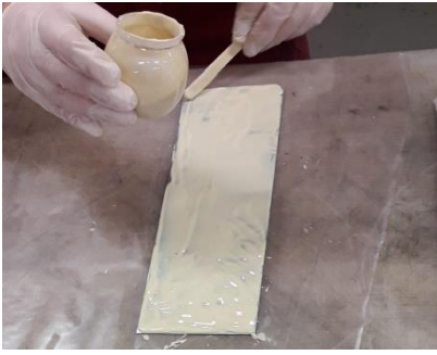
Figure 44 Adhesive applied into the metal sheet
