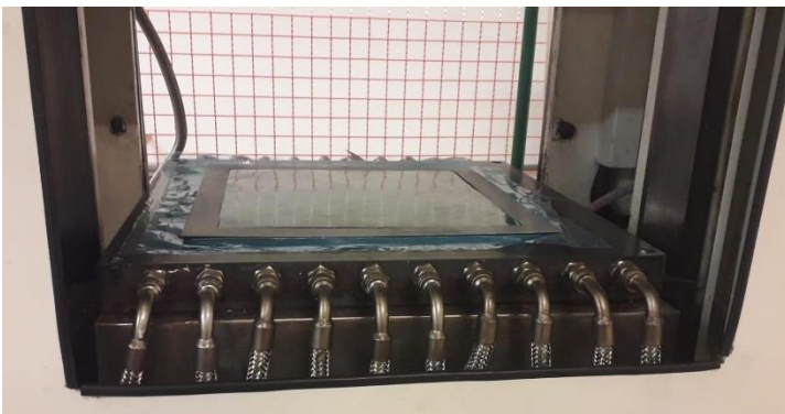
Figure 36 Left: before starting the cure, the skins are place inside the hot press; Right: during the cure process
