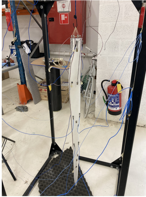
Figure 4.16: Experimental setup for the hammer test.
