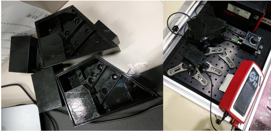
Figure 68 - First version of the prototype, produced using Polyjet technology.
