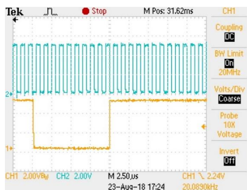
Figure 3.9 - Data message and clock detailing that each data bit lasts ten clock cycles.
