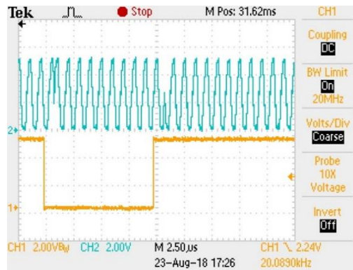
Figure 3.10 - Oscilloscope results showing the BPSK modulated waveform according with the binary message data.
