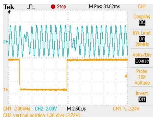
Figure 3.12 - Oscilloscope results showing the current waveform on the transmitter coil.
