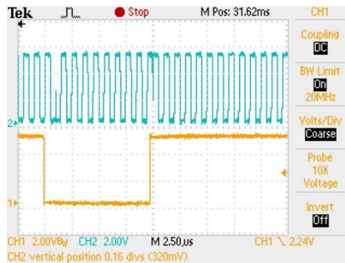
Figure 3.11 - Oscilloscope results regarding V_{\text{drain}} on Class D PA.
