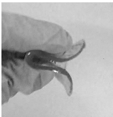
Figure 6.21. Flexibility of cured film obtained with Resin B.
