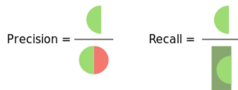
Figure 3.10: Recall and precision as seen from 3.9 in a binary classification scenario. Adapted from [Wik18].
