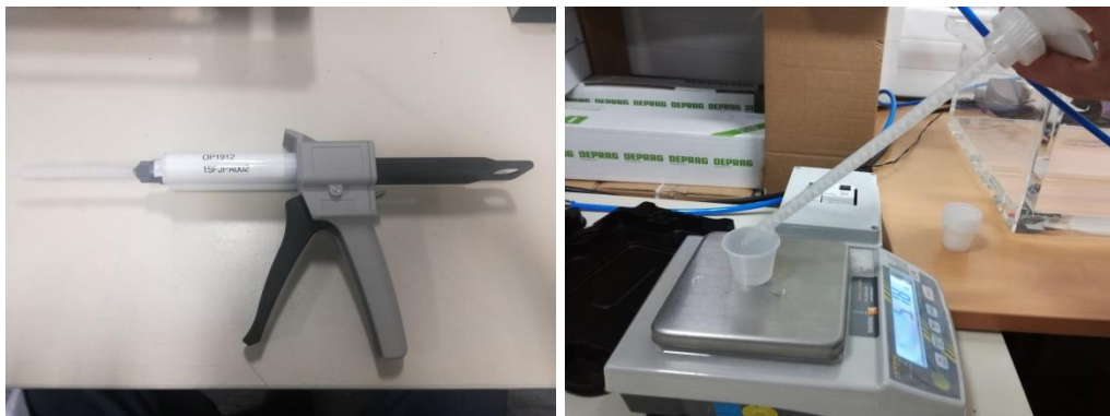
Figure 18 – Manual dispenser of OB with static mixer (left); Quantity measurement of OB in scale (right)
