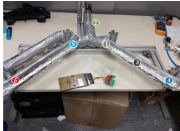
Figure 29 - Termopile of OCS version 1 with potentiometer of heater set in level 2 scheme of instrumentation The same test was conducted for the 6 level of the potentiometer which represents maximum power of the heater, working continuously for around 30 mins to access if the problem persists. The result is shown in Figure 30 and its nomenclature is:
