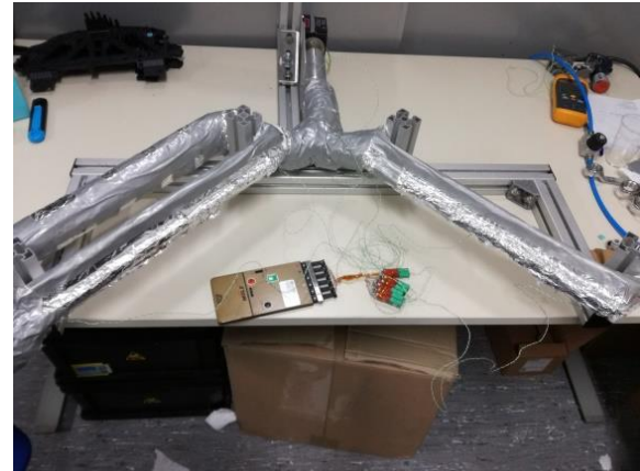
Figure 30 - Thermoprofile of OCS version 1 with potentiometer of heater set in level 6 scheme of instrumentation
