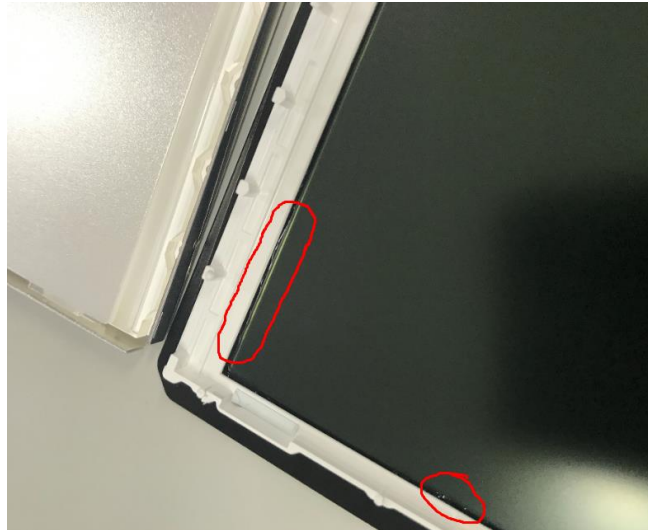
Figure 2 – Infiltration of LOCA in the interior of the display
