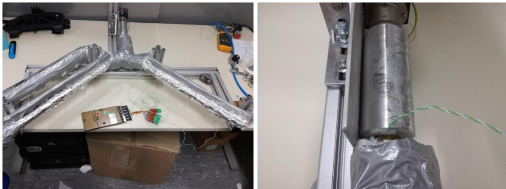
Figure 27 – Instrumented system (left); Termopair in heater nozzle (right)
