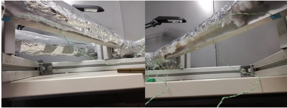
Figure 28 – Two termopairs in left air curtain (left); Three termopairs in right air curtain (right)
