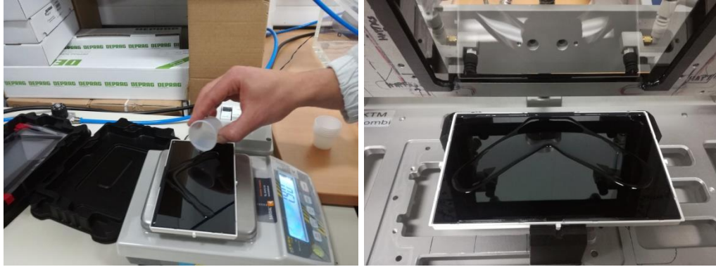
Figure 19 – Dispensing of OB material in display (left); Manual assembly jig opened with display and cover layers (right)
