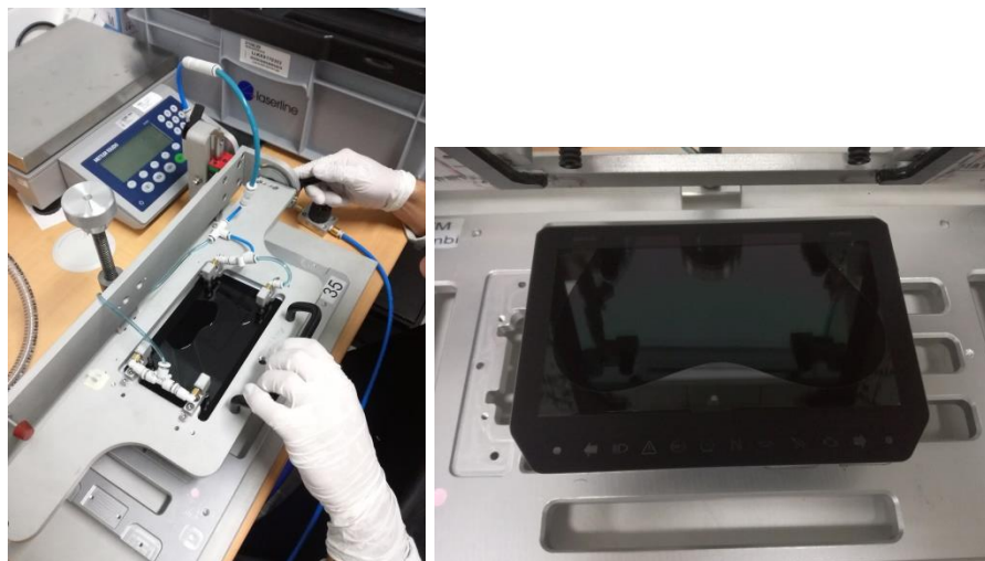
Figure 20- Assembly of both layers until 1st point of contact (left); Spreading of Optical Bonding after releasing glass layer (right)
