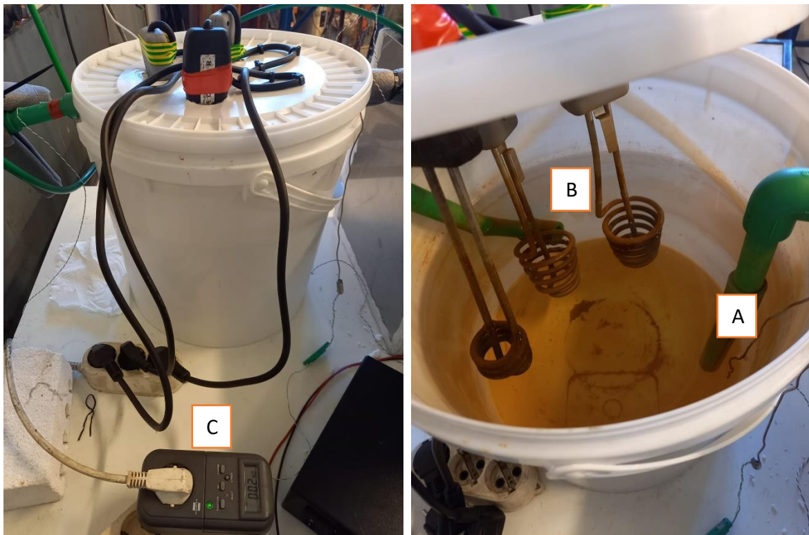
Figure 3.5 – Heating process. A – Probe; B – The three resistances; C – Watt meter.
