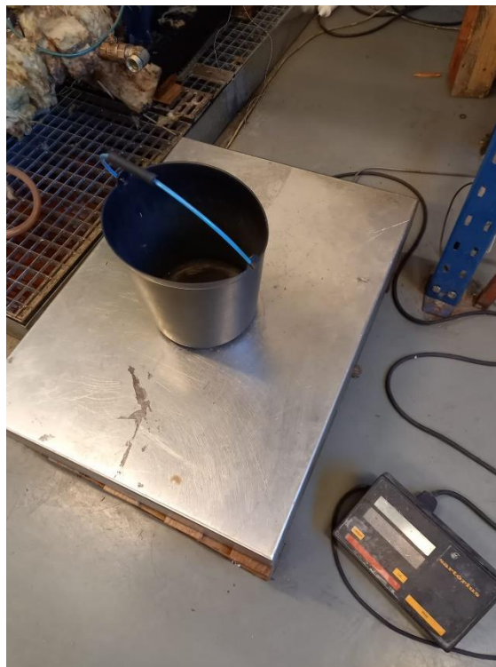
Figure B.1 – Weighting scale used in the calibration of the flow meters.
