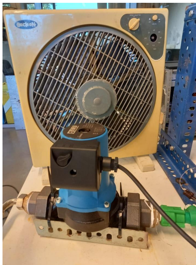
Figure 3.4 – Pump with the cooling fan.
