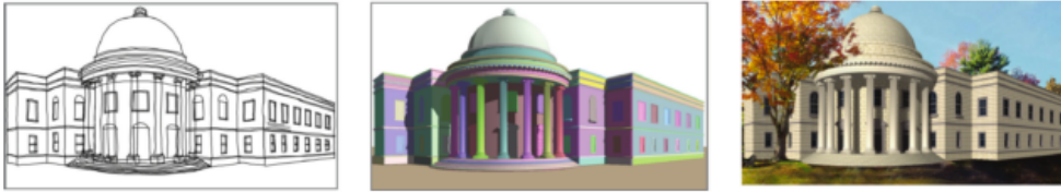
Figure 3.6: From a single user sketch (left) the system extracts the building structure (centre) and provides a detailed textured result (right) [Che+08b].
