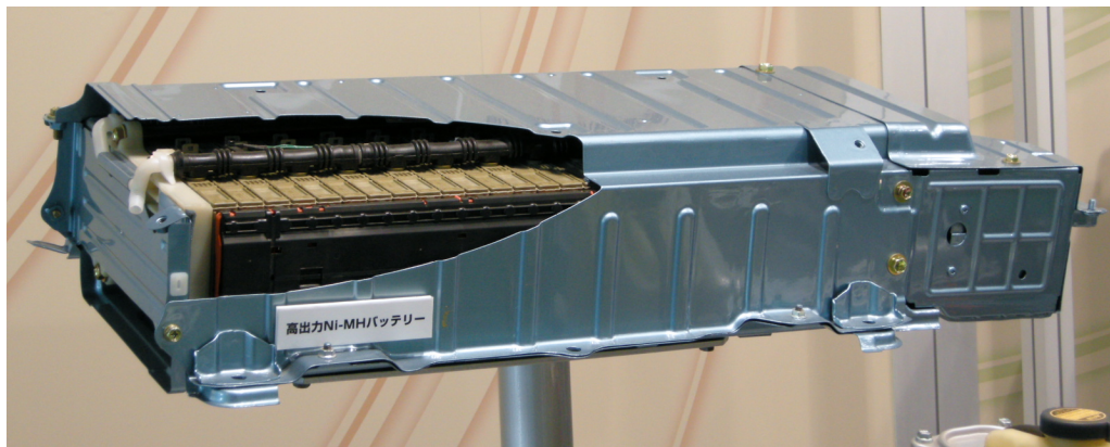
Figure 2.5: The high-power NiMH battery of a Toyota Prius. Figure taken from [4]
