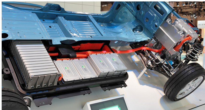
Figure 2.6: Nissan Leaf's Li-ion battery pack. Figure taken from. Table [5]
