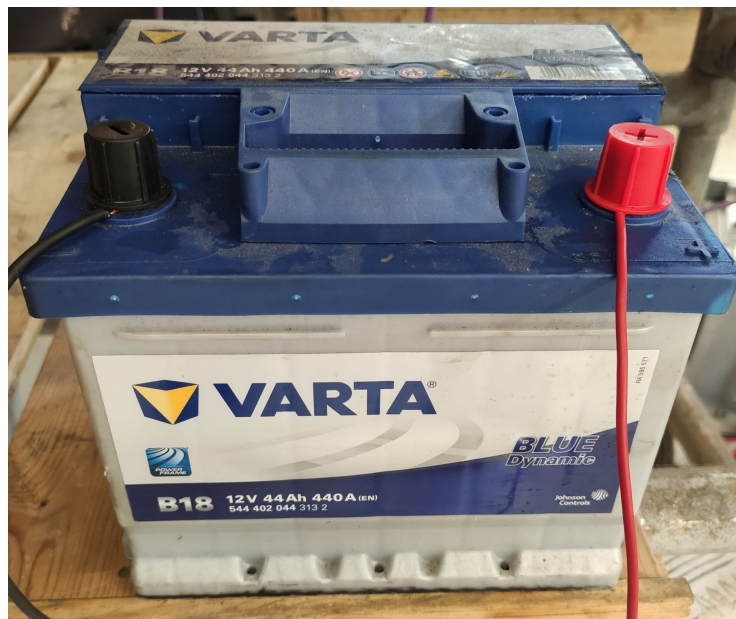
Figure 2.4: Lead-Acid Battery from Varta
