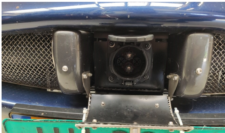
Figure 3.10: CHAdeMO socket for fast charging
