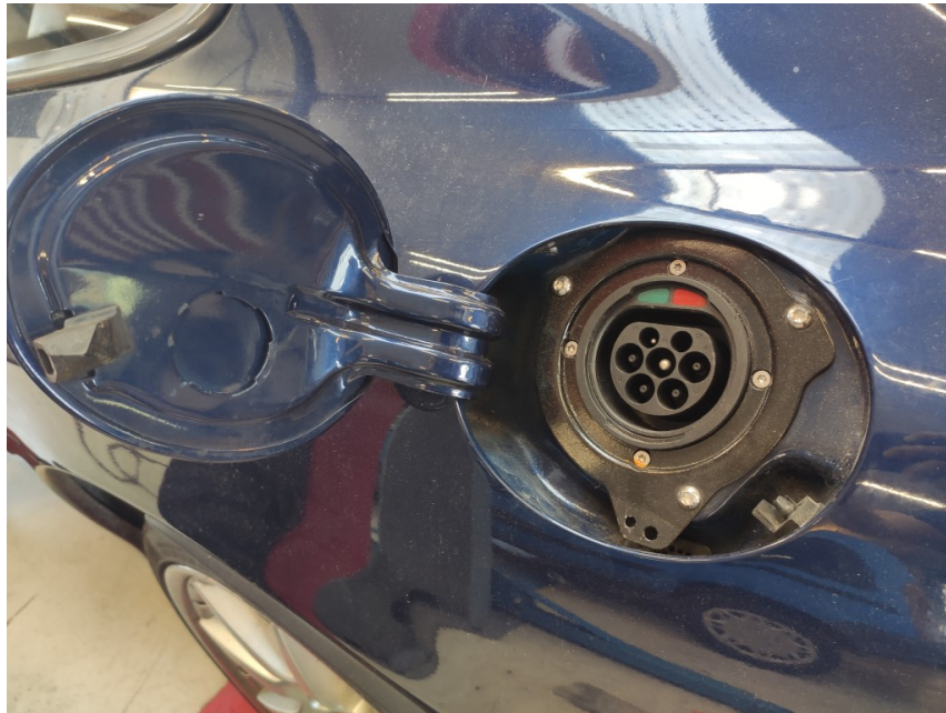
Figure 3.9: Type 2 socket, for AC charging
