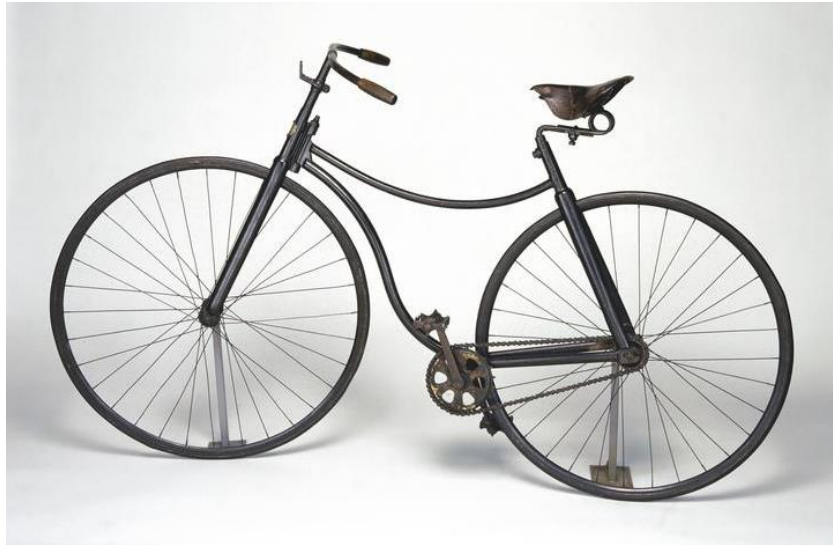
Figure 4 – The Rover ‘Safety’ bicycle, c. 1885. Source Science Museum Group Collection, 27/05/2021, ( https://collection.sciencemuseumgroup.org.uk/objects/co25833/rover-safety-bicycle-1885-bicycle ).
