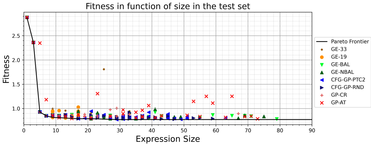
Figure 6.5: Fitness and size of the non-dominated DRs and the best DRs of the 20 runs in the test set. It is also represented the DRs belonging to the Pareto frontier of all algorithms.
