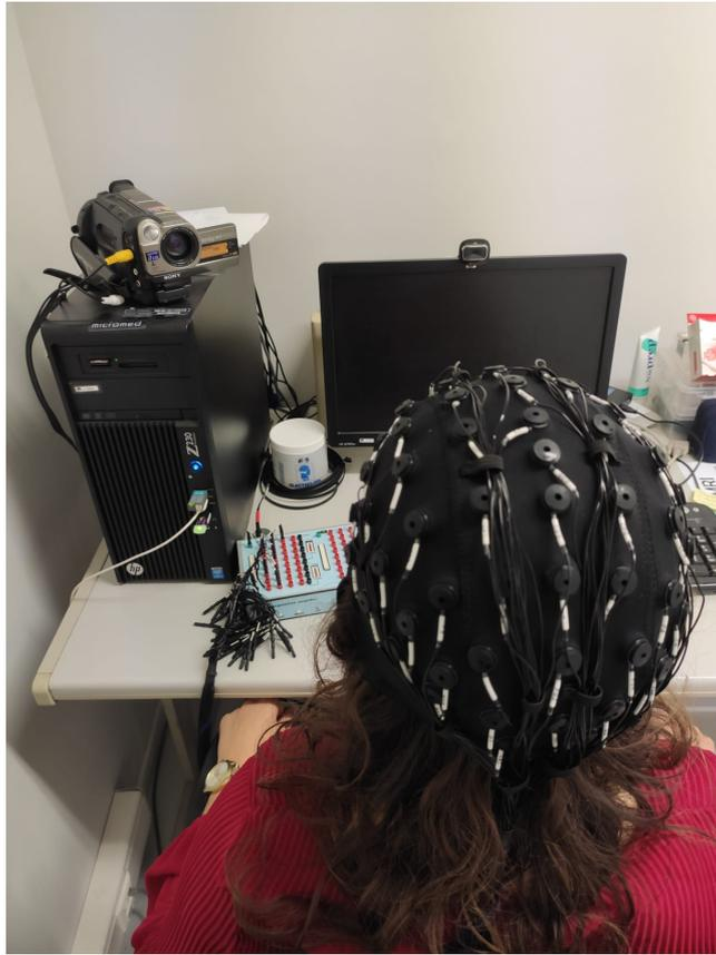
Figure 4.1: Photograph of the experimental setup used to study movement with EEG signals in healthy subjects.
