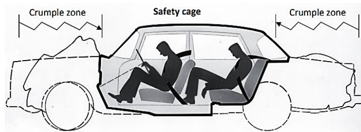
Figure 3- Scheme of the basic car zones regarding safety functions (Zhao and Jiang 2017).
