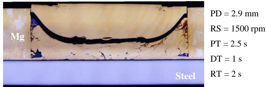
Figure 82- Cross-sectional macrostructure of SZ pull-out defect.
