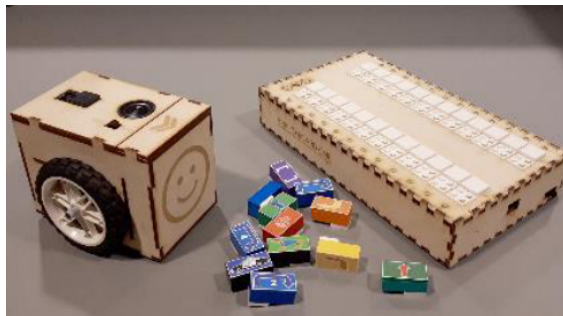
Figure 2.16: BRICKO educational robot and its programming board.
