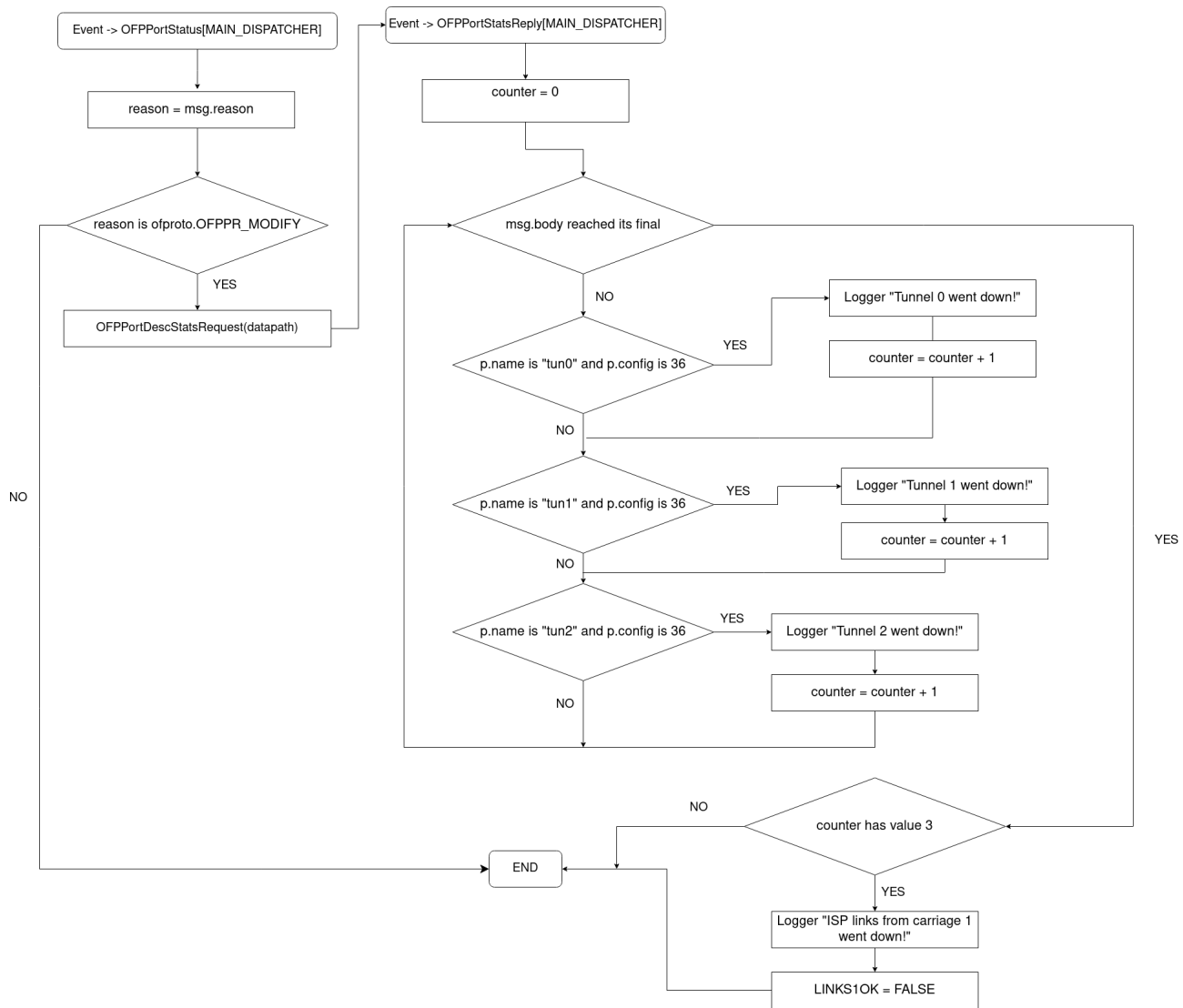
Figure 3.28: OFP OFPPortDescStatsRequest and OFPPortDescStatsReply interaction flowchart.
