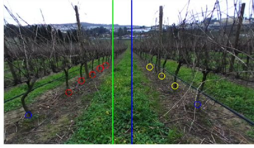
Figure 3.8: Horizontal error, green line is the measured average horizontal distance between the selected points (blue circles).
