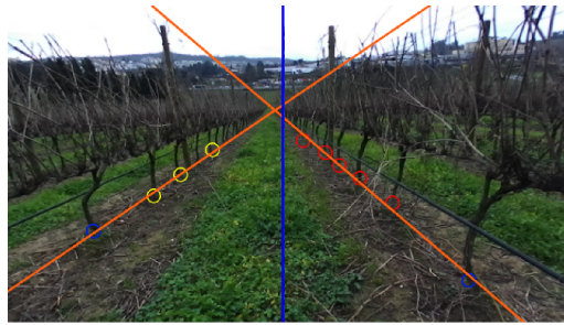
Figure 3.6: Linear approximation step, the blue line is the center of the image, the orange lines represent the best fit calculated for each row.
