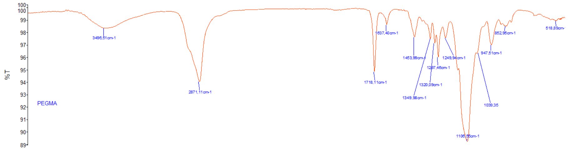
Figure A. 4. Fourier transform infrared spectrogram of PEGMA. Notice the main peaks at 2871, 1250, 1718 and 1106 cm -1 .
