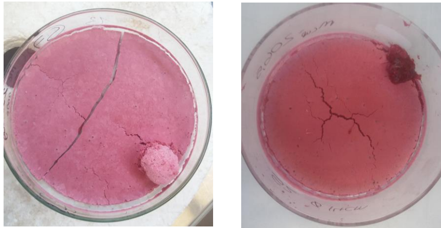
Figure G 1 - Foam collapsing (hot spots) caused by microwave freeze-drying.
