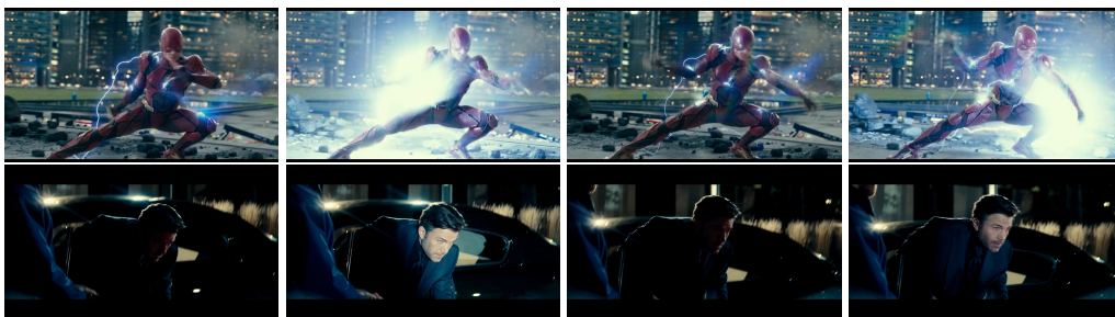
Figure 5.8: Fast consecutive changes in color information, specially brightness, leads to the incorrect detection of multiple shot boundaries
