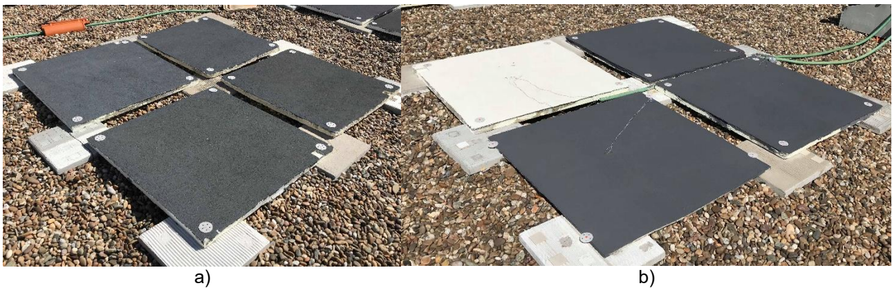
Figure 2: Analysed specimens: a) 3-years ageing; b) 2-years ageing (excepting the white specimen).
