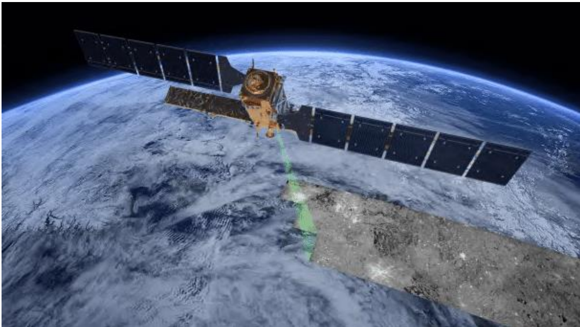
Figure 1: Illustration of a space-borne SAR sensor. Source:(Raab, 2016)
