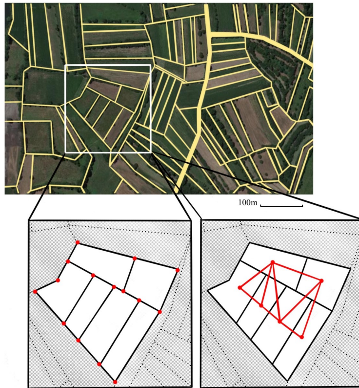
Figure 2.2: Plot layout. On the left: abstraction of lots as polygons; On the right: abstraction of lots as nodes
