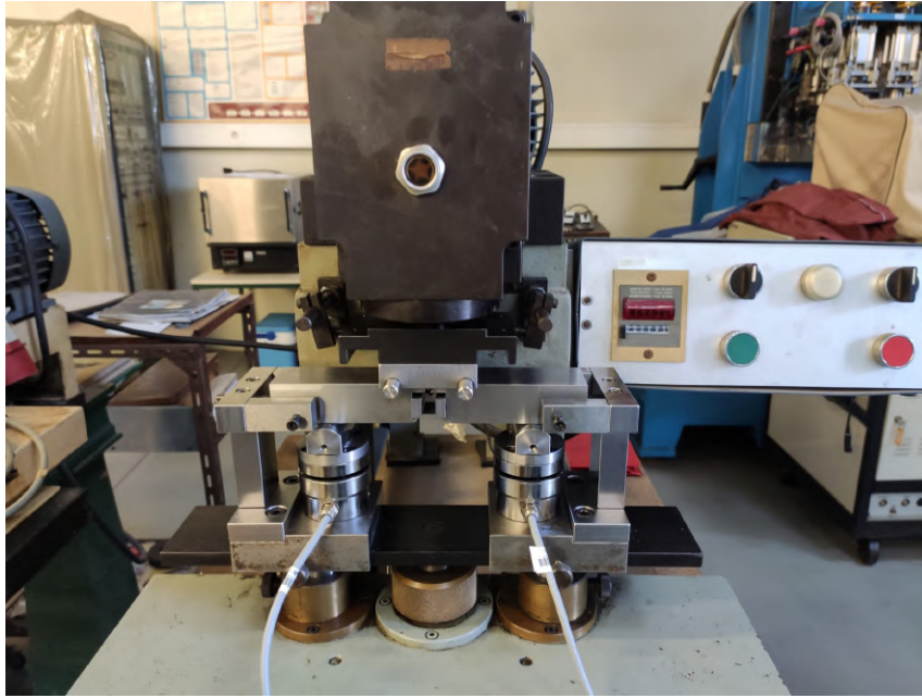
Figure 3.36: Miniature specimen testing machine with adequate gripping system.
