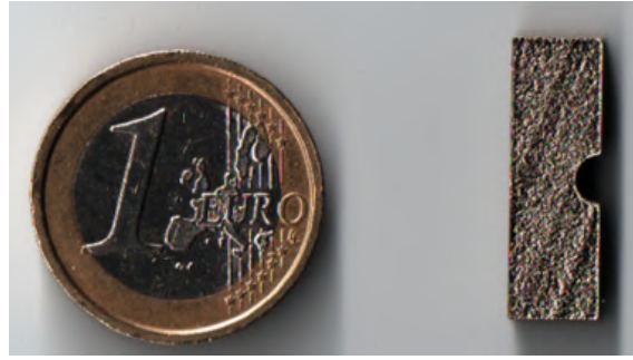
Figure 2.48: Fatigue testing miniature specimen proposed by Nicoletto, with a size of ( 7 \times 5 \times 22 \text{ mm}^3 ). One euro coin as size reference [63].
