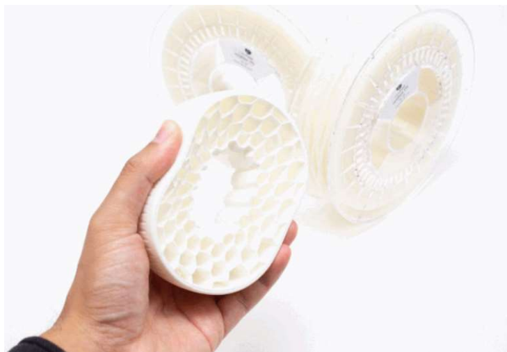
Figura 12 - soft touch characteristics of varioShore TPU.
