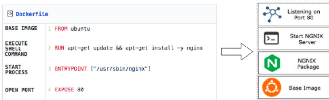
Figure 3.1: Basic dockerfile for a NGINX Server and its 4 goals
