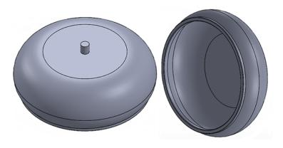
Figure 5.7: Model of the Kiwi suction cup in 3D, obtained using SOLIDWORKS software.
