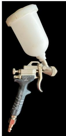
Figure 3.6: HVLP gravity feed air spray gun used in the experimental trials.
