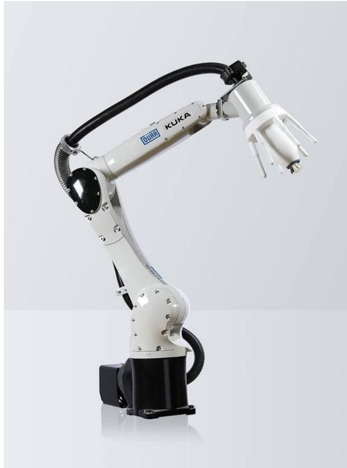
Figure 2.3: KUKA ready to spray package [3].
