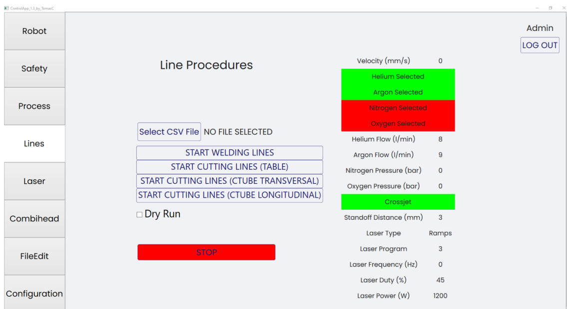
Figure 4.11: Display of the MainWindow - "Lines" Tab
