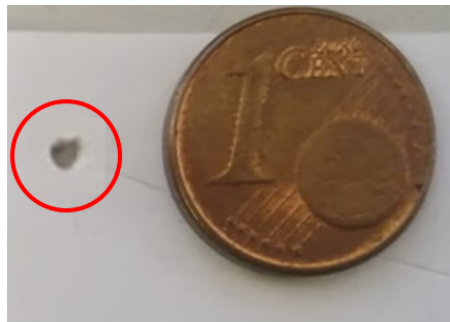
Figure 5.1: Results from the laser system test with a 30ms discharge
