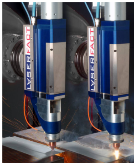
Figure 3.8: Combi-head F2Y laser cutting (left) and laser welding (right) of metal sheets [32]
