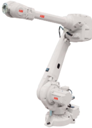
Figure 3.1: ABB IRB 4600 40kg 2,55m [22]
