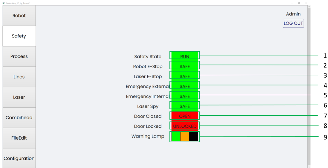
Figure B.7: Components of the MainWindow - "Safety" Tab
