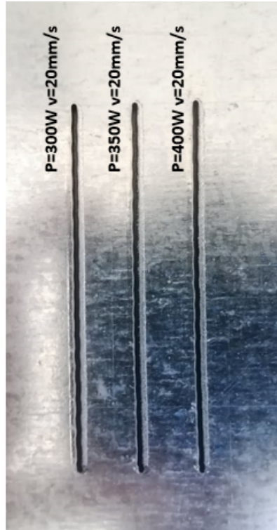
Figure 5.9: Results from the second line test - horizontal lines with new path
