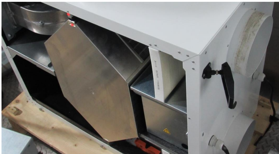
Figure 5.10 – Heat Recovery Ventilation system.
