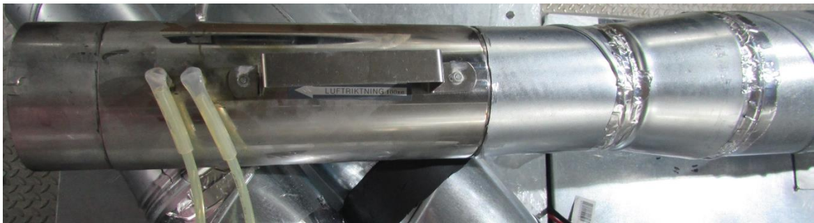
Figure 5.5 – Volume flow rate measurement device.
