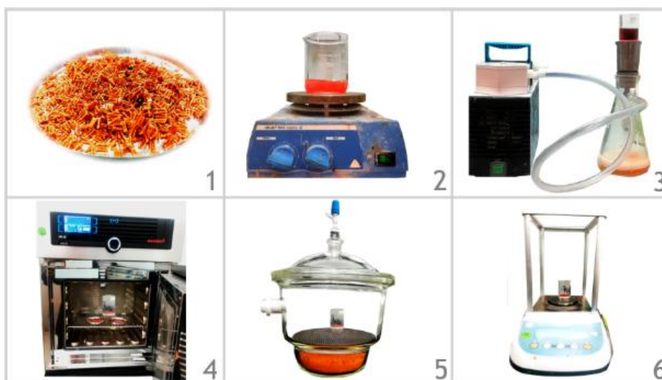
Figure 13 - DIP measurement via wet chemical method for nylon textiles.
