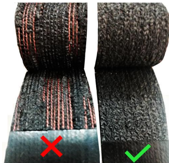
Figure 7 - Peel adhesion results
