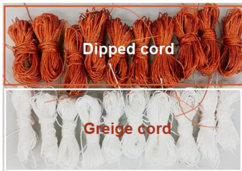
Figure 12 - Samples used in the weighing method.
