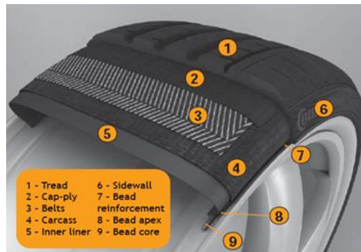
Figure 1 - Example of the tire constitution (adapted from Continental, 2013).
