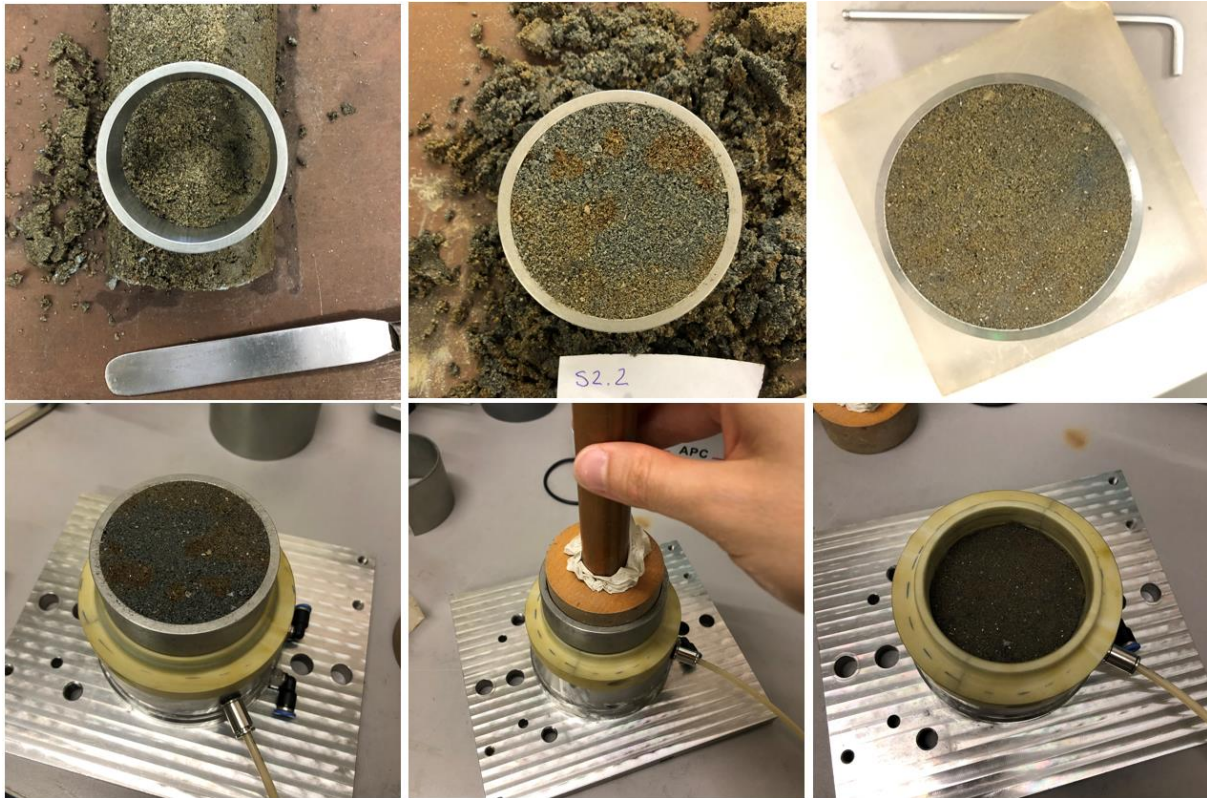
Figure 6.20 – Sample preparation of an undisturbed specimen for simple shear tests
