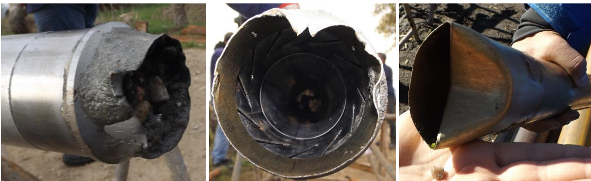
Figure 3.27 – Gel-Push core catcher and D&M liner damage
