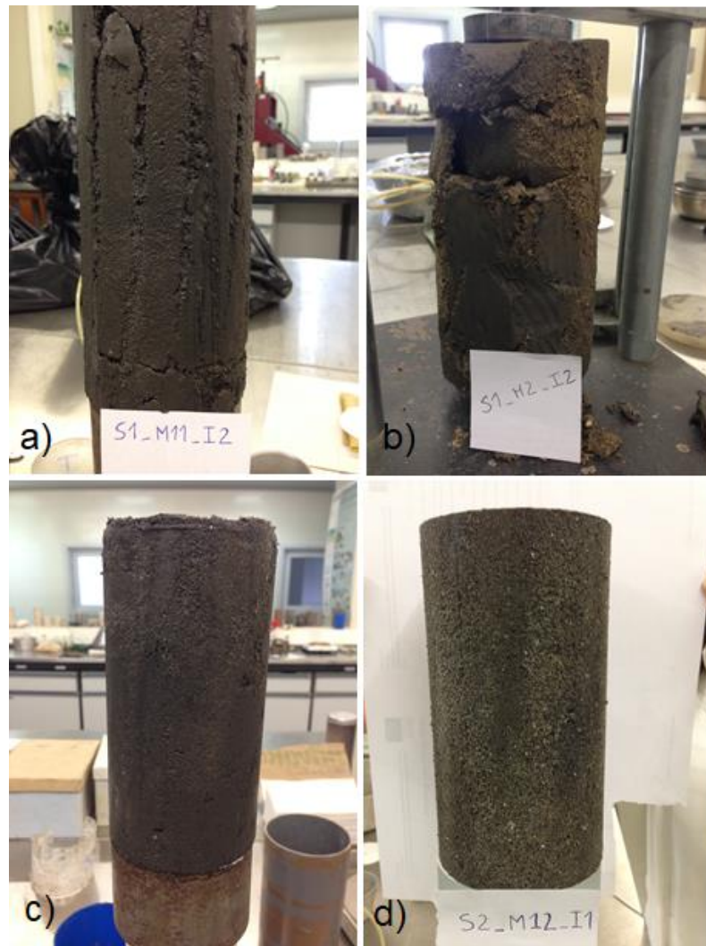
Figure 5.1 – Samples collected with Mazier sampler: a) and b) samples with damaged surface; c) and d) homogeneous samples adequate for triaxial testing
