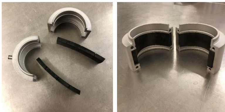
Figure A.3– Adaptation of the mould to prepare specimens without rings
