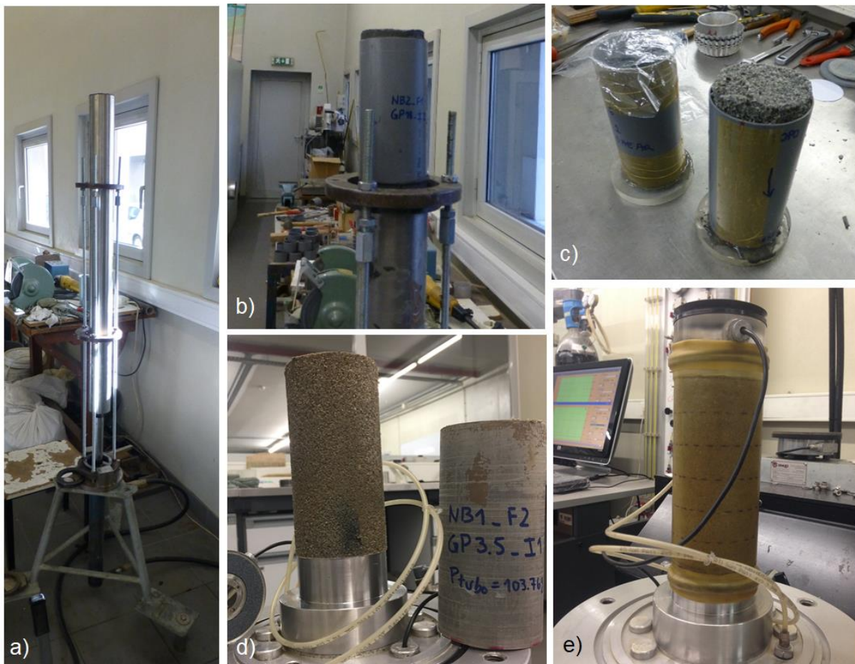
Figure 6.17 – Gel-Push sample preparation procedure: a) hydraulic extractor; b) extraction of specimen; c) preparation of smaller specimen for storage; d) assemblage on the triaxial cell; e) specimen ready for triaxial test
