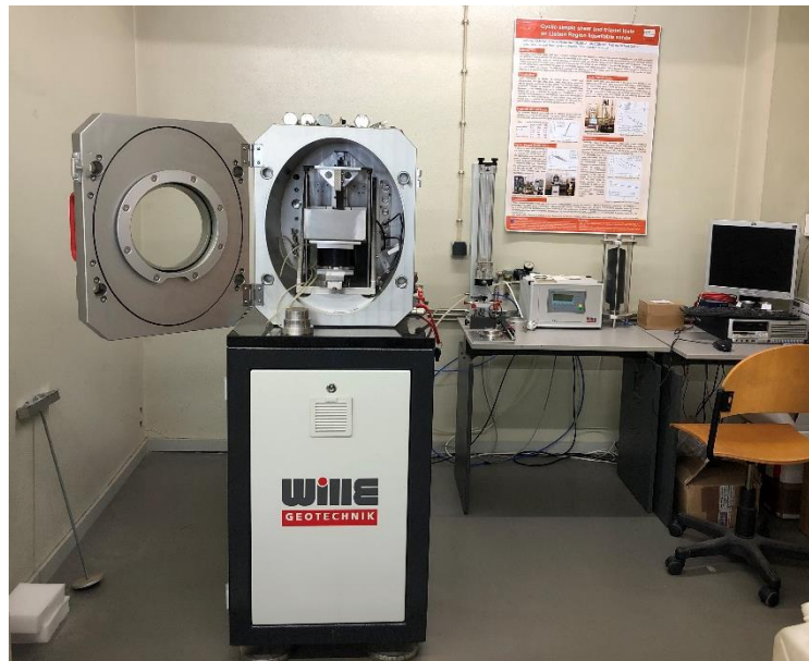
Figure 6.12 – Cyclic simple shear equipment at FEUP
