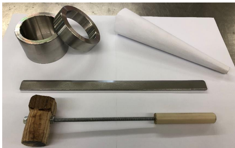
Figure 6.5 – Equipment used for the determination of maximum and minimum soil densities
