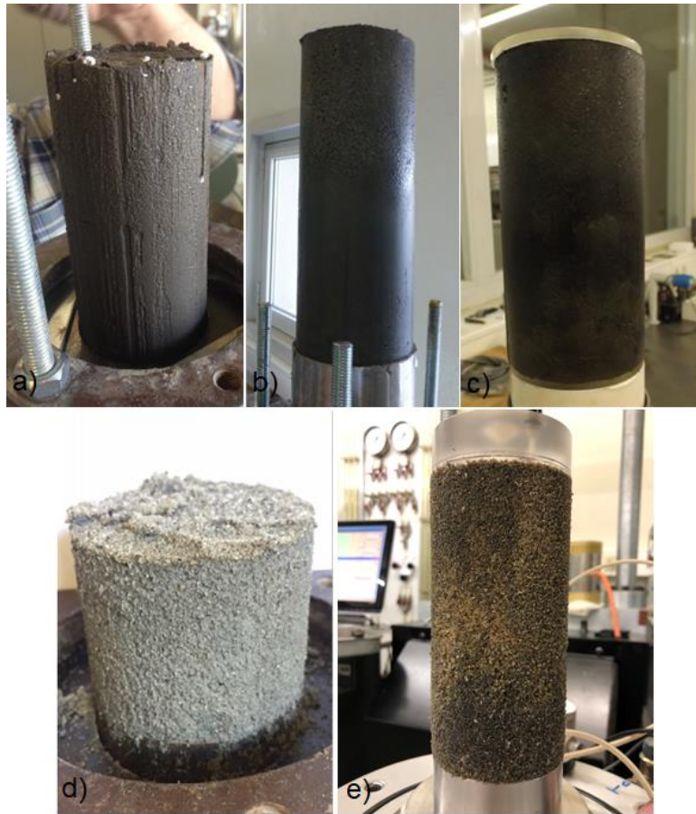
Figure 5.2 – Samples extracted from GP sampling tubes: a) clay sample; b) and c) silty sand samples; d) and e) sand samples
