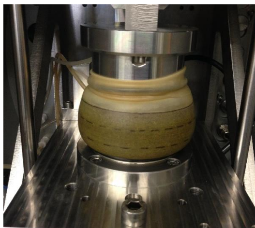
Figure A.18 – Shape of the specimen after applying the vertical stress
