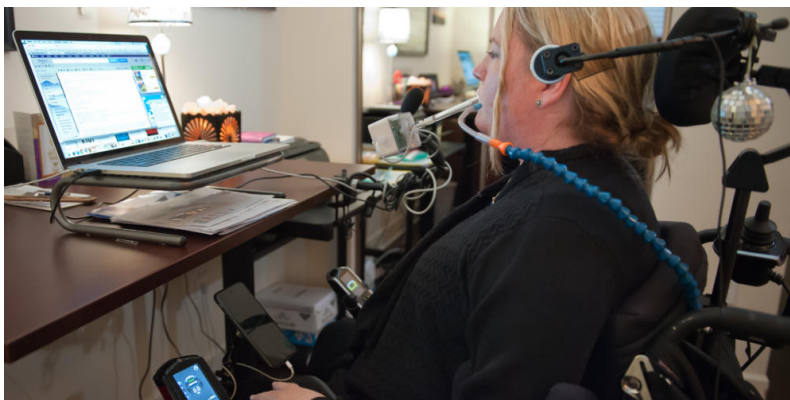
Figure 3.1: Example of mouth stick use for operation of a computer (extracted from [50]).
