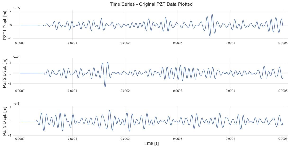
Figure 12: Representation of a random aluminium plate test, with a signal from each of the 3 PZT sensors. Hole size = 2 mm; Hole position (x,y) = (194,209) mm.
