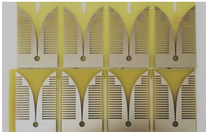
Figure 3.23: Fitting cutouts for the antennas.
