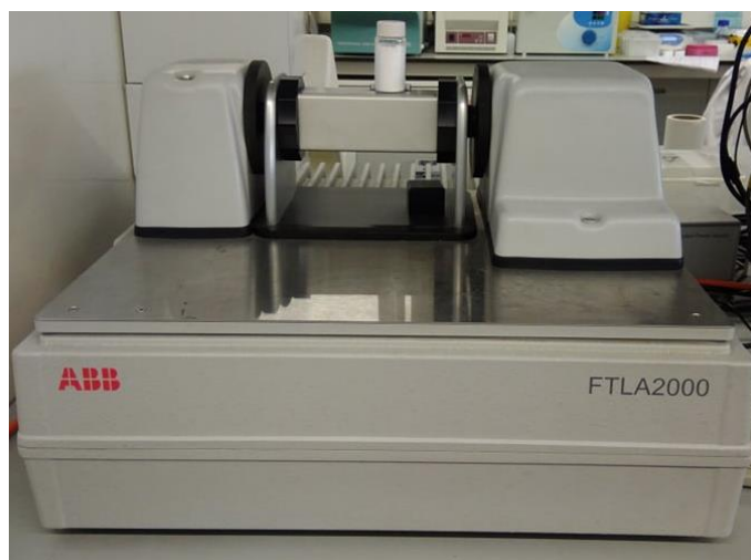
Figure 15: FT-NIR equipment with sample placed in the accessory of powder measurement (FTLA2000, ABB).
