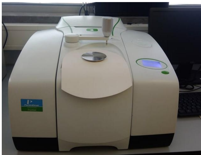
Figure 14: FT-MIR equipment with ATR accessory (Frontier, PerkinElmer), where samples are directly placed, pressed with a pressure element and measure.
