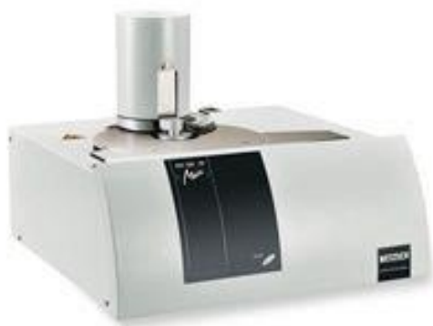
Figure 17: DSC equipment with autosampler accessory (DSC 200 F3 Maia®, Netzsch-Gerätebau GmbH).
