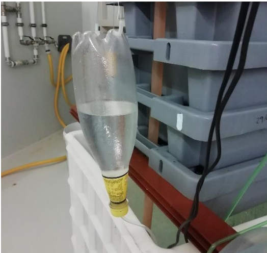
Figure 24 - Ammonium chloride solution container.
