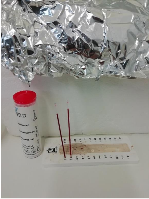
Figure S10 - Capillary tubes filled with blood samples, capillary tube support and plasticine.
