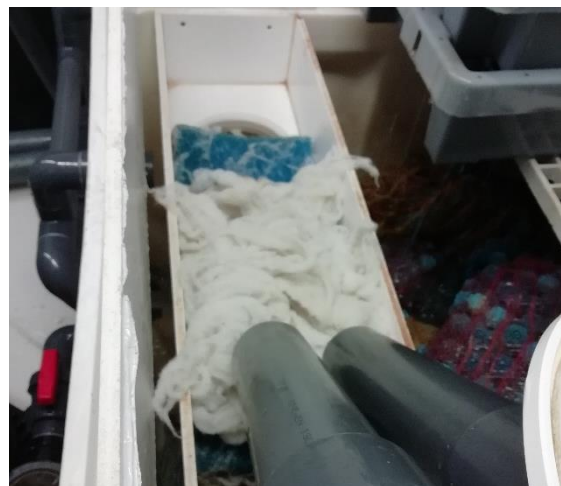
Figure 10 - Mechanical filters - glass wool (white); sponge (blue).
