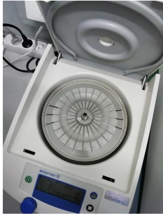
Figure S11 - Haematocrit centrifuge with capillary tubes after centrifugation.
