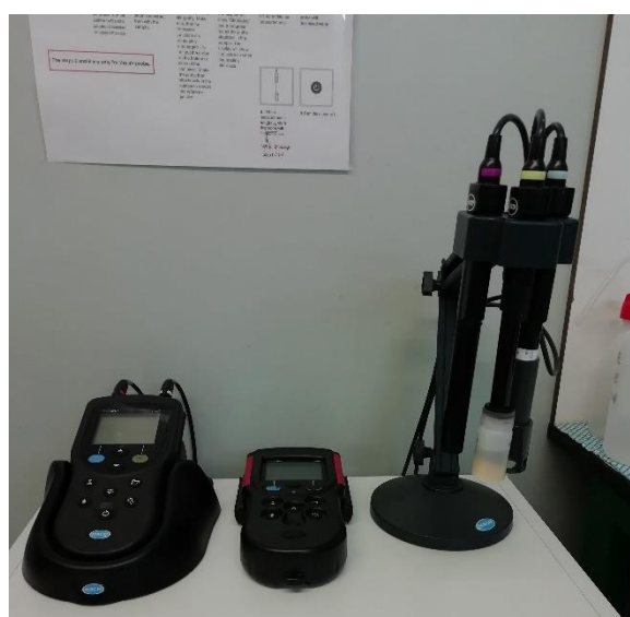
Figure 2 - Salinity (left), pH (centre) and dissolved oxygen (right) probes in BOGA's sampling room.
