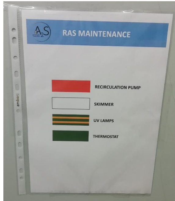
Figure 41 - Identification code for the electric plugs in challenge room p.14.
