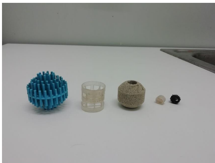
Figure 12 - Different types of filter media ("Bioballs") used in BOGA.
