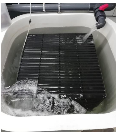
Figure 13 - Submerged flow-through biofilter in BOGA (down-flowing).
