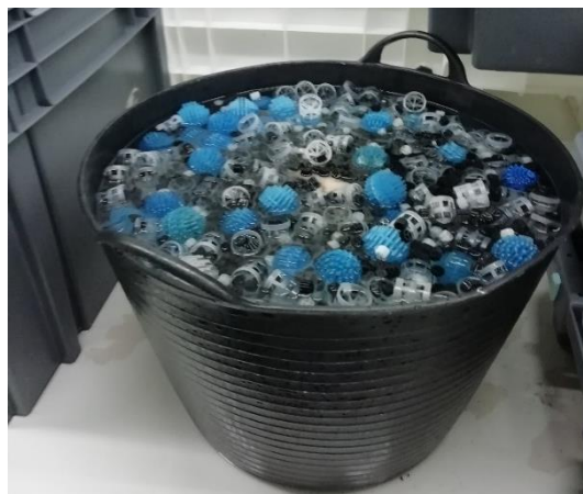
Figure 26 - Container with filter medium undergoing disinfection.
