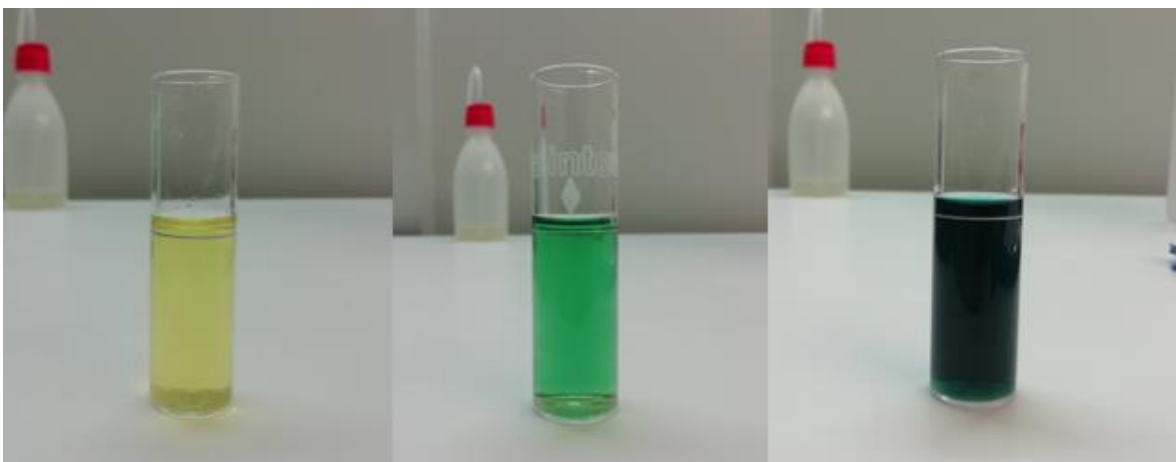
Figure S6 - Colour change in samples with progressively higher concentrations of ammonia (left to right).
