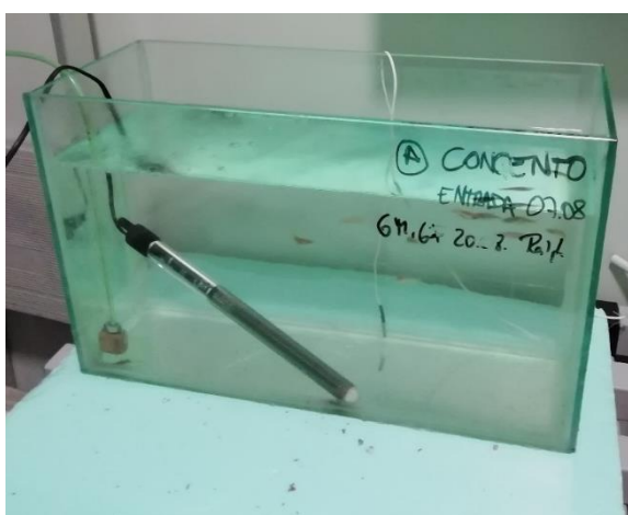
Figure 20 - Submersible heater used in BOGA.
