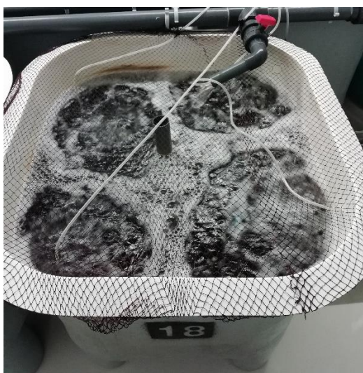
Figure 30 - Tank in aquaculture room p.20 used as a fluidized biofilter.
