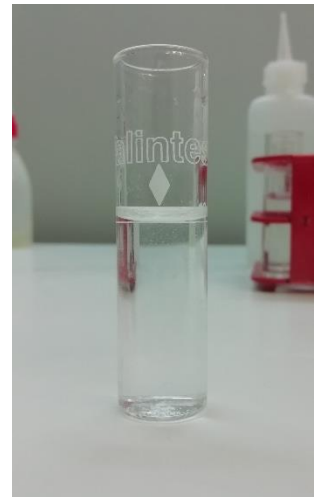
Figure S5 - Sample for ammonia measuring with sufficient conditioning reagent.
