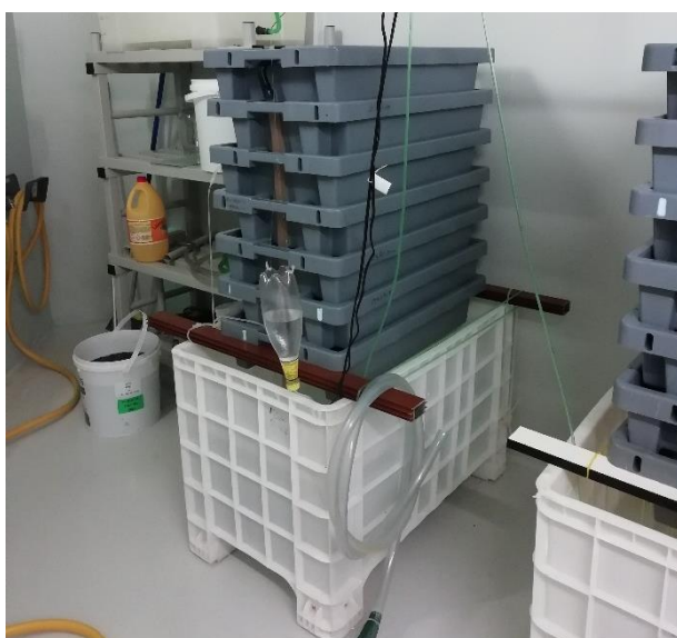
Figure 22 - Freshwater biofilter activation system.
