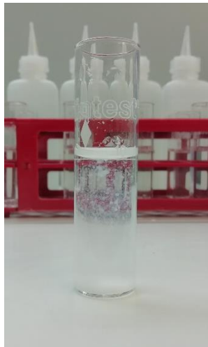
Figure S4 - Sample for ammonia measuring with insufficient conditioning reagent.
