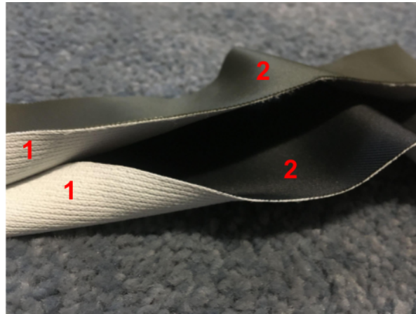
Captions: 1 - PET layer (9% of the material weight); 2 - PVC layer (91% of the material weight).
