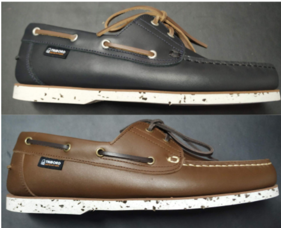
Figure 5.2: Leather shoe model with an outsole with 5% leather (top) and another one with 10% leather (bottom).
