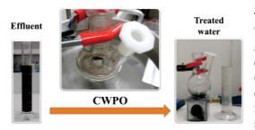
Figure 2. Color removal during the CWPO run performed at pH 6 and in situ magnetic separation system employed for catalyst recovery after the reaction stage.
