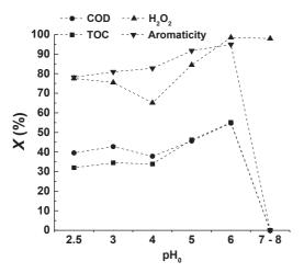
**Figure 1.** Chemical oxygen demand (COD), total organic carbon (TOC), hydrogen peroxide (H<sub>2</sub>O<sub>2</sub>) and aromaticity conversions obtained in CWPO runs performed during 24 h with CoFe<sub>2</sub>O<sub>4</sub>/MGNC (0.5 g L<sup>-1</sup>) and T = 80 °C.
